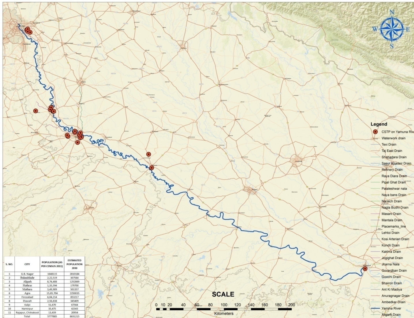
Fig : 3.2, GIS map showing STPs and drain of River Yamuna
